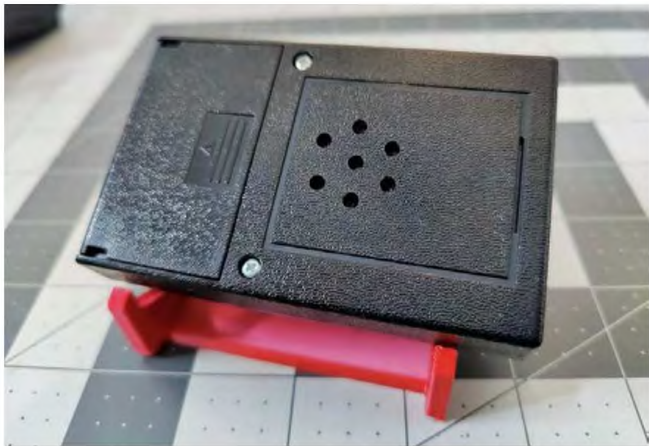
Figure 5 — A view showcasing the back of the CW Elmer, which contains a rear-firing speaker and cover that houses a 9 V battery (not included).
