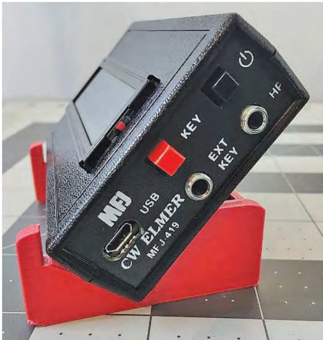
Figure 6 — A side view of the MFJ-419 CW Elmer includes a micro-USB port for power or for use with a terminal client, such as Tera Term . A power button controls if the unit is on or off. An external key port allows the user to use their own straight key while practicing Morse code but also allows practicing Morse code with no key, by utilizing the red KEY button. The KEY button can also act to navigate through the menus. Finally, an HP port allows the user to use the CW Elmer with headphones for better hearing or to be considerate of others in the area.
